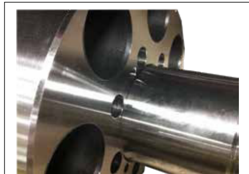
5. Place where shaft is screwed into barrel
