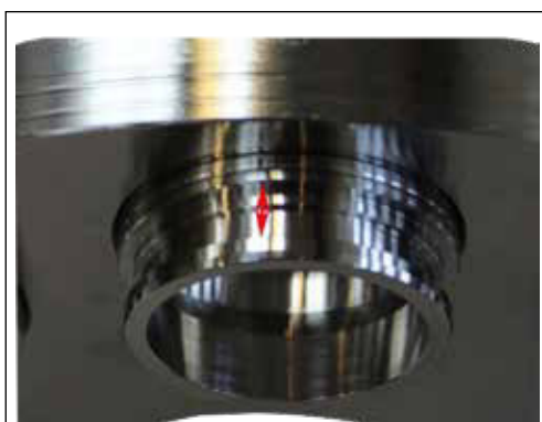
1. Valve plate (thrust pad, close-up)
