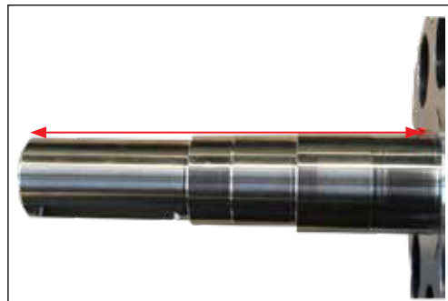
3. Cylinder barrel (shaft surface)
