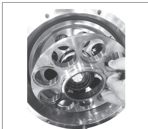
11. Remove the retainer plate.
