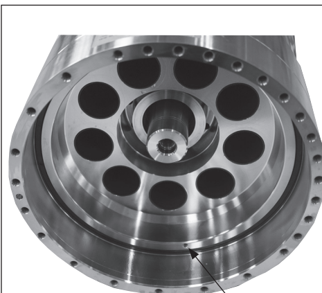
26. Screw 2 M6 x 65 screws in the cylinder barrel.
