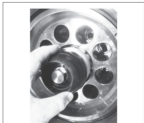
12. Remove the retainer ball.
