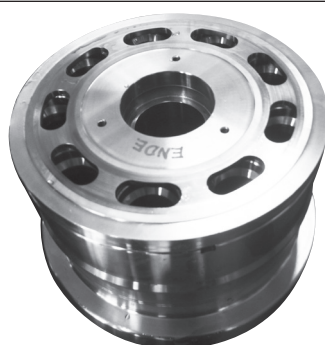
28. Remove the 2 M6 x 65 screws and place the cylinder barrel on a clean surface with the valve plate on top. For more information on how to disassemble the valve plate assembly, please see the section "Disassembling and assembling of the valve plate".
