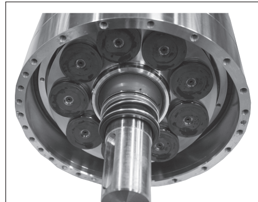
20. Remove the motor flange following the same steps described for the end flange (steps 2 to 9). Using the M8 x 140 mm is optional.
