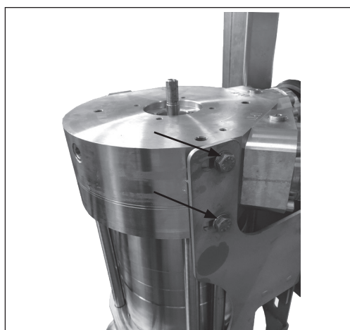
7. Mount the four M 10 bolts in the bracket in the motor flange tighten to 45 Nm using 17 mm socket.
