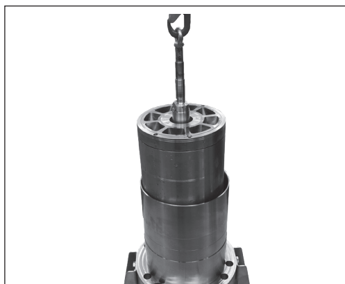
13. Mount the M6 lifting eye on the cylinder barrel big shaft end and carefully lower the cylinder barrel straight into the housing. Afterwards remove the lifting eye.
