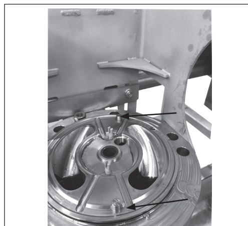
16. Be careful when lifting the port plate off the port flange to keep the two pins in the port flange.
