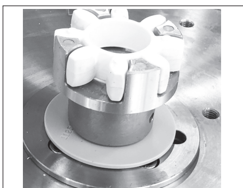
34. Lubricate the shaft. Mount the dust cap onto shaft. Mount key. Mount the coupling onto the shaft all the way down to the dust cap and press down for tight contact. Tighten the screw inside the coupling to 2 Nm using a 4 mm Allen key. Mount the spider.
