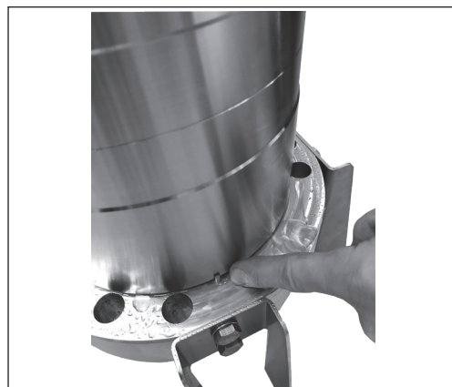
12. Install the housing onto the port flange: Check that the new pin is still placed in the port flange and place the hole for the pin in the housing carefully over the pin.
