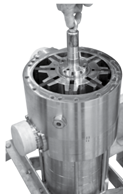
2. Carefully lower the rotor straight into the stator housing, internal coupling and green spider.
