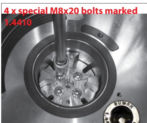
27. Unscrew the four special M8x20 bolts marked 1.4410. using the 6 mm allen socket.
