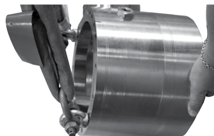
34. Unscrew the stud bolts using a 6 mm allen key to avoid the stud bolts get bended before placing the stator housing horizontally.
