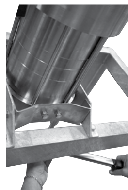
32. Remove the nuts and washers (the stud bolts may get loose and fall down).
