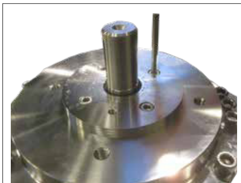
17. Lubricate the screws. Mount a new O-ring on the shaft cover and mount it on the motor flange. Tighten the screws to the torque according to exploded view.
