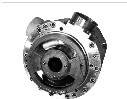
35. Unscrew and remove the lifting eyes and lifting strap and turn the stator housing up so that the port plate is upwards to avoid damage.
