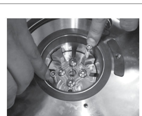
28. Remove the coupling from the cylinder shaft. If sticking, screw in 2 x M5 bolts (not in tool kit) which will allow a better grip to pull out the coupling.
