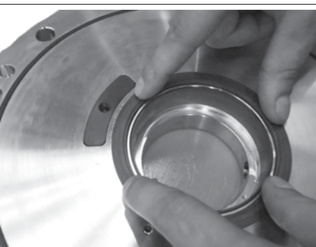
15. Carefully by hand only press down the side plate. Always change rotor stop and side plate at the same time as changing the rotor elements.
