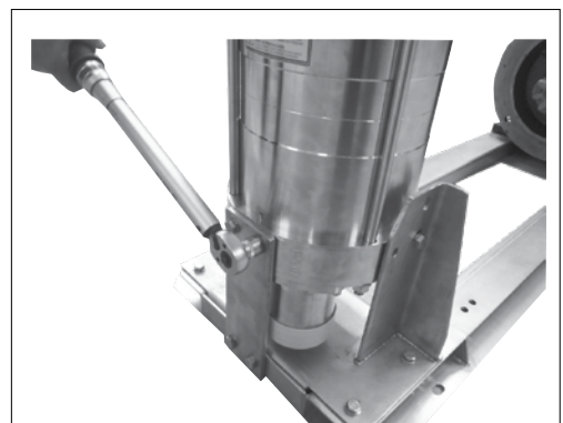
14. Tighten the screws with 30Nm..
