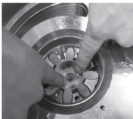
9. Mount the green spider inside the internal coupling.
