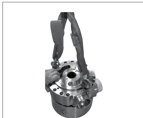
41. Mount 2 lifting eyes across from each other in the intermediate flange to equal the weight and use a lifting strap to lift the flange away from the stator housing.
