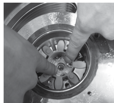
26. Remove the green spider from the internal coupling.
