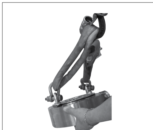
42. Remove the lifting eyes and strap and place the intermediate flange with the bearings side upwards.
