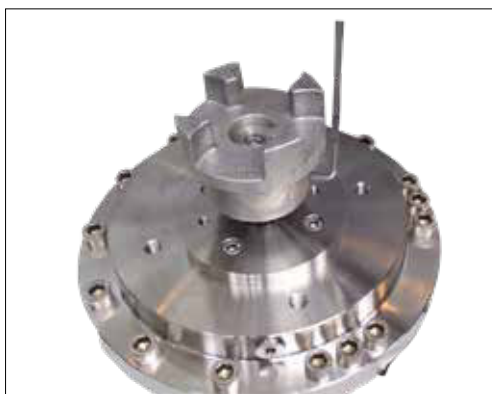
19. Tighten the screw inside the coupling to the torque according to exploded view.
