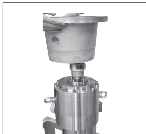
20. Mount the spider and the bell housing over the shaft seal cover outside diameter.
