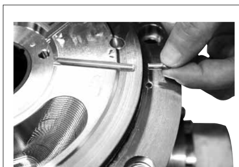
39. Remove the small pin for fixing the exchanger housing in the intermediate flange.
