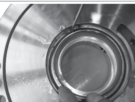
13. Mount the second new O-ring in the bottom on the flange.
